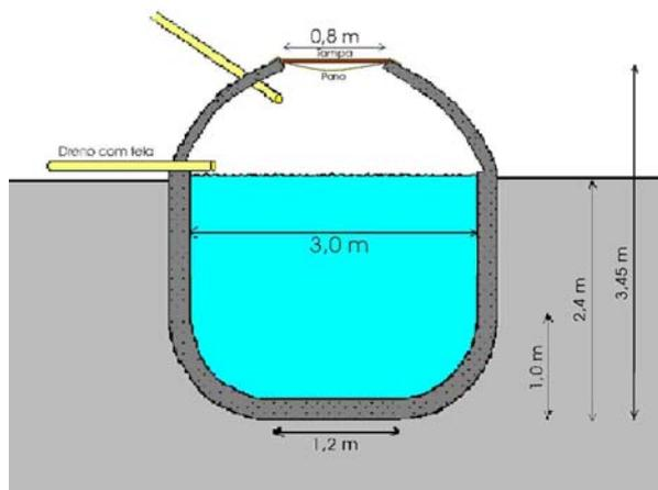
Illustration 8: Cross-cut of lime and bricks cistern (10 000 l)
