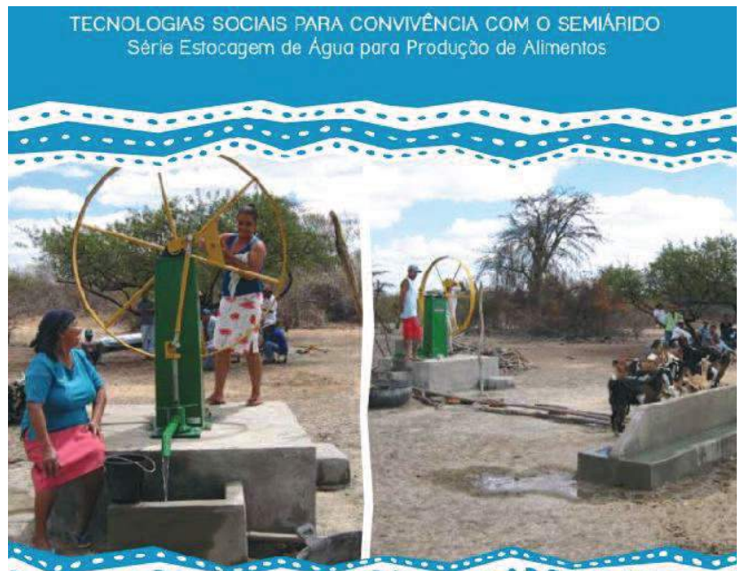
Figure 6 The Bomba d'Água Popular, based on the Volanta design (ASA)
